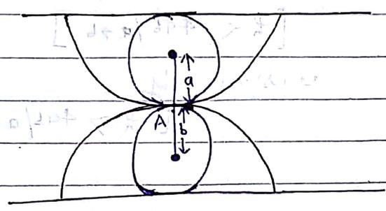
Intrinsic equation of the cycloid is given by  $S = 4a \sin \psi$
