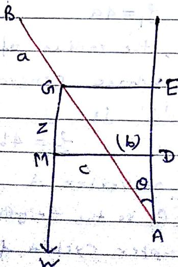
Let AB be a uniform rod of length  $2a$ . The end A of the rod rests against a smooth vertical wall and the rod rests on a smooth peg C, whose distance from the wall is say  $CD = b$
